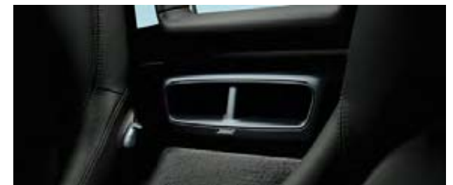
Active subwoofer enclosure with 5.12-inch (13.0-cm) low-range speaker and 2.52-inch (6.4-cm) high-/midrange speaker
