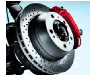
Standard disc and caliper (Boxster S)
