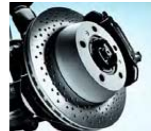
Standard disc and caliper (Boxster)
